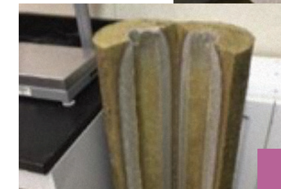
Stone wool after high temp exposure
