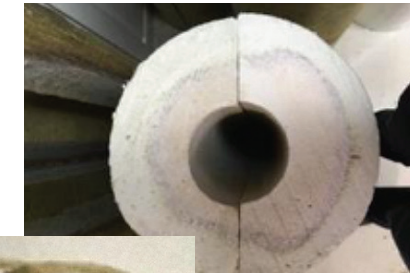
Calcium silicate after high temp exposure
